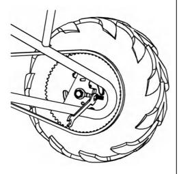
5. Tighten chain adjusters using 12 mm wrench evenly to remove some slack from the chain as required.
