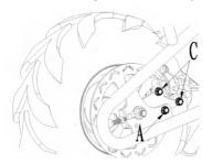
Chain and Sprocket Notes: The chain will typically have a "loosespot" and "tight spot" corresponding with a sprocket rotational position. This is normal and common to all chain-driven products due to run-out tolerances
