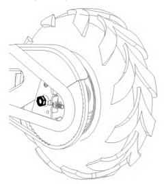
Replacing the chain requires removal of a Master Link. Removing outer retainer allows this link to be removed. Be careful not to damage clip. Note. Install clip as shown
