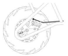
8. Tighten the brake mount plate bolts (A) and (C) securely. Re-attach the chain guard. Test ride. Readjust as needed.
