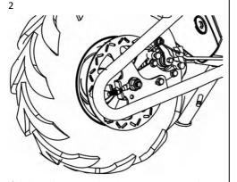
If the brake has too much slack, use a 10 mm wrench to loosen the brake anchor cable for additional adjustment.
