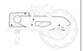
2. With a 5mm Hex Key wrench remove Brake Mounting Plate adjuster screw (A). Loosen the brake cable anchor bolt and remove cable (B) If replacing tire also remove 2 Brake caliper mounting bolts (C) and remove caliper.
